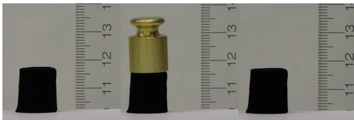
Figure 3.9. A 3_{\text{annealed II}} SWCNT aerogel (left, 17.4 mg, density: 9.8 mg/cm 3 ); the same sample supporting a 20 g weight (middle, ~1150 times its own weight); the same sample after removal of the weight (right).
